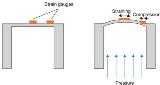
**Figure 2:** Deflection of the sensor diaphragm under pressure
