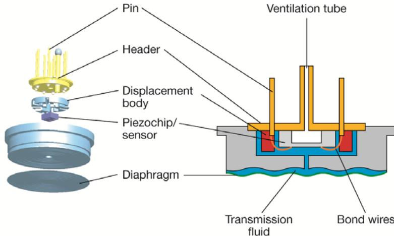
**Figure 8:** Design of an encapsulated piezo-resistive sensor
