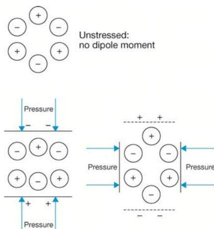
**Figure 4:** Piezo-electric effect
