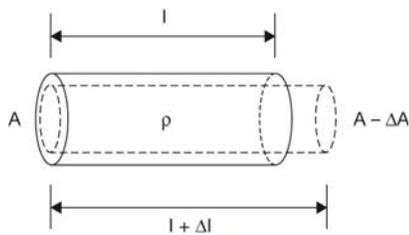
**Figure 1:** Change of the dimensions of a cylindrical conductor by elongation
