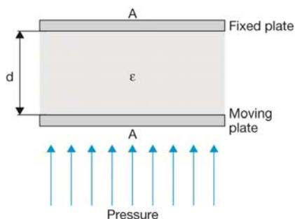
**Figure 3:** Capacitive measuring principle
