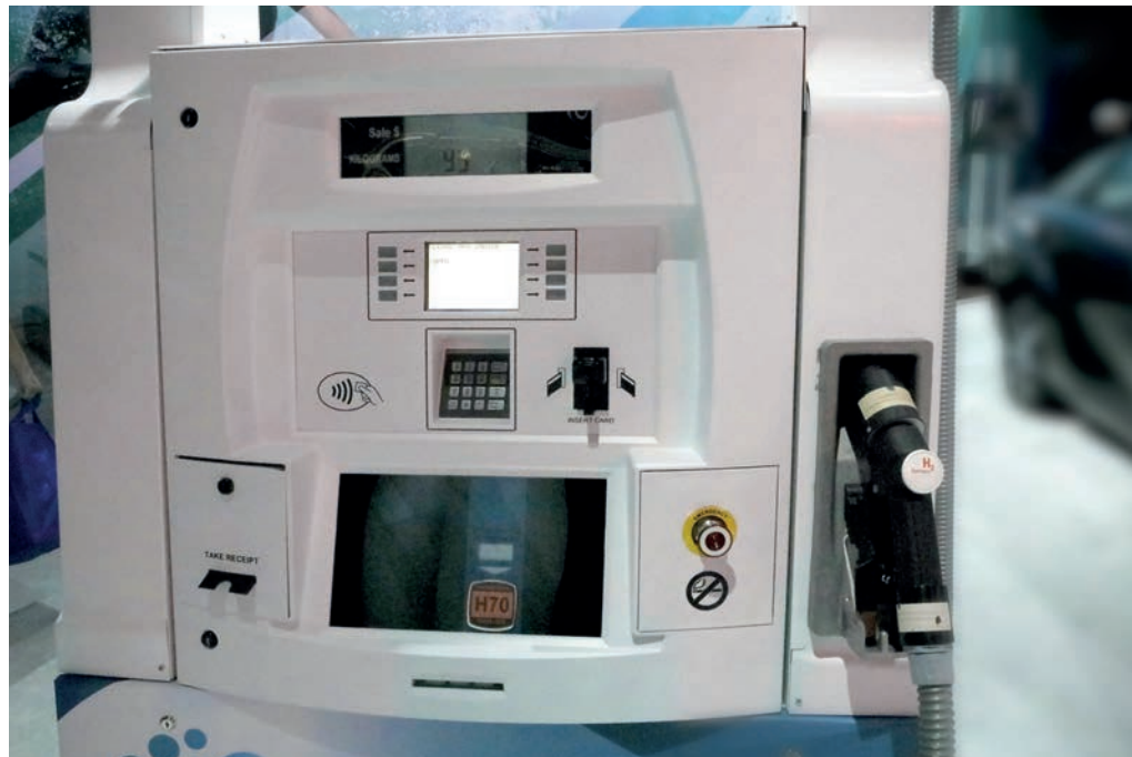
The measuring solutions in the H 2 refuelling process must work reliably over a long period at pressures of up to 900 bar and temperatures from -40°C to +85°C ©: istockphoto
