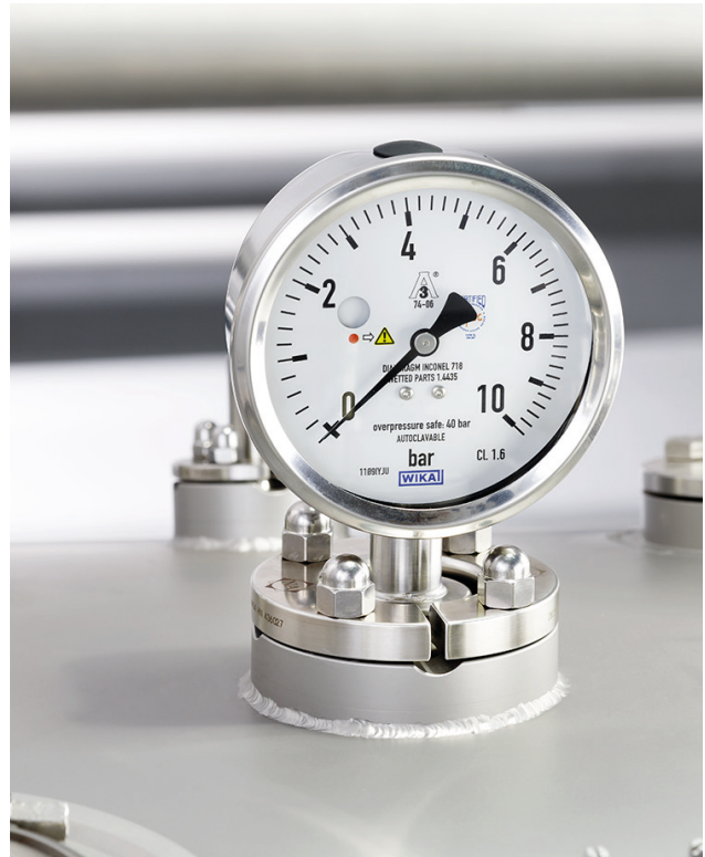
WIKA PG43SA-D flush diaphragm pressure gauge made of stainless steel, and with a hygienic process connection for sterile process technology.
