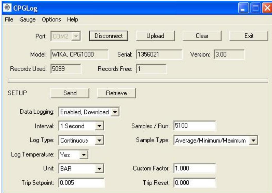
The top portion of the display contains controls to connect to a gauge, disconnect from a gauge, upload logged data, clear logged data, and exit the application. Once connected to a gauge, it shows the model, serial number, and firmware version of the gauge, plus the number of data logging records presently used and free.
