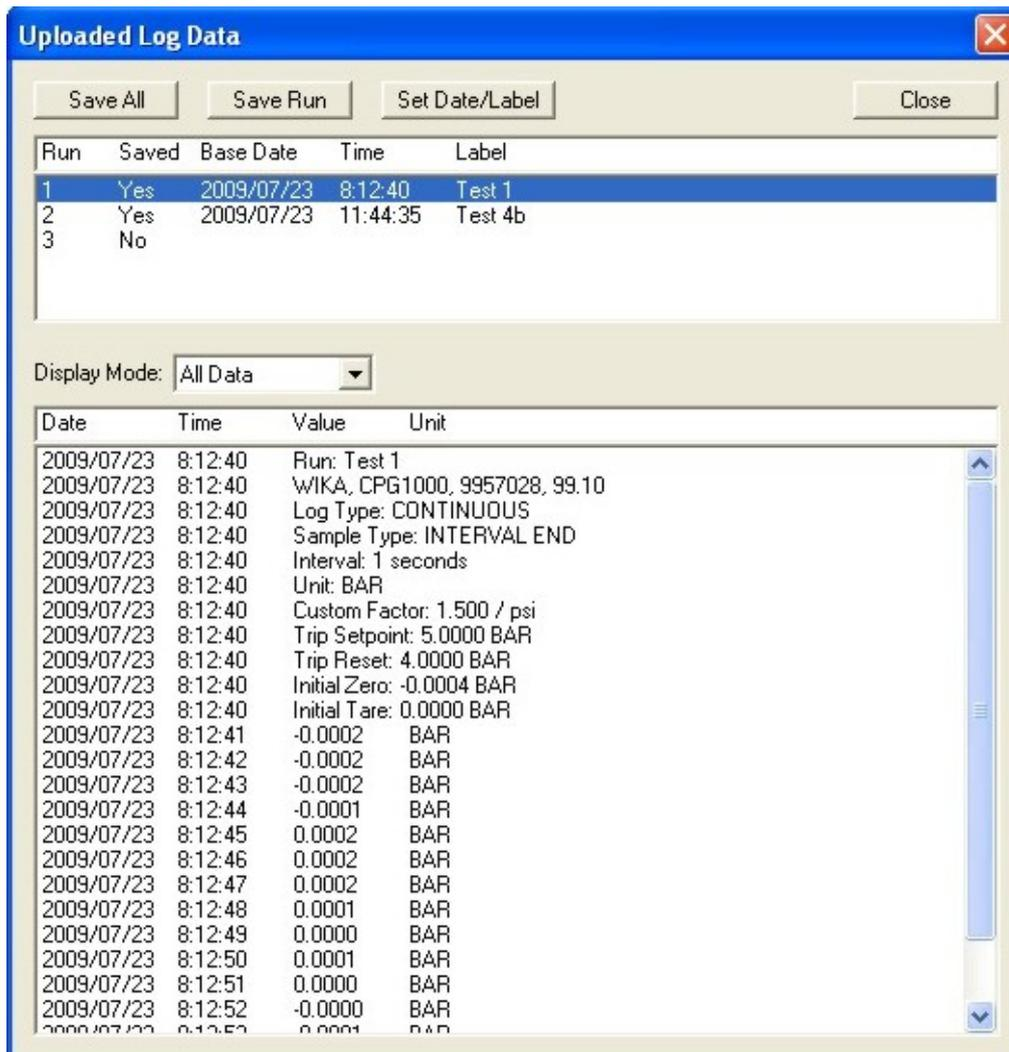
The top portion of the display lists the individual data logging runs found in the uploaded data. To display a run's data in the lower portion of the display, highlight it by clicking on it. Use the Display Mode box to select the subset of run data displayed: All Data, Selected Data, or Readings Only. When the Display Mode is set to Selected Data, click the Change Selection button to modify the display options. This is described further under Display Options in section 4.5.
