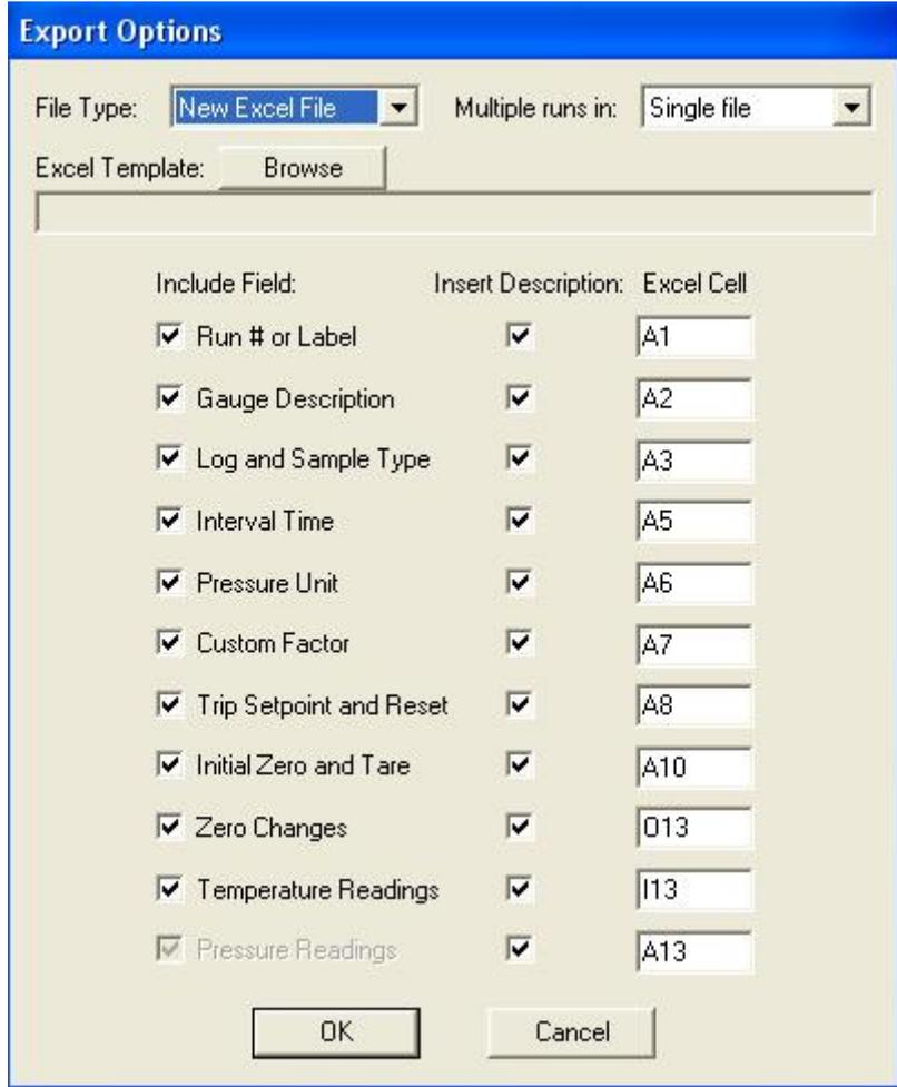
This screen is used to modify the default selections for the file type and run description fields to be exported from the Log Upload Display. When data is initially uploaded the selections are set to these default values. After the initial data display, the selections may be temporarily changed for each export operation, and remain changed for the duration of the data display. Logged pressure readings are always exported.
