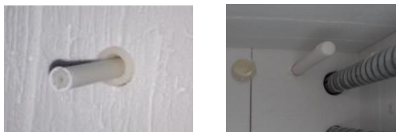
Fig.2: a) Mounted sensor prototype b) Embedded TC and heating coils
