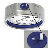
Before reading the pressure, tap the case lightly to release friction in the movement and ensure a precise indication.
