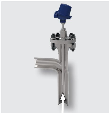
The insertion length and the diameter of the thermowell are dependent on the process conditions, especially on the flow rate of the measured medium.
