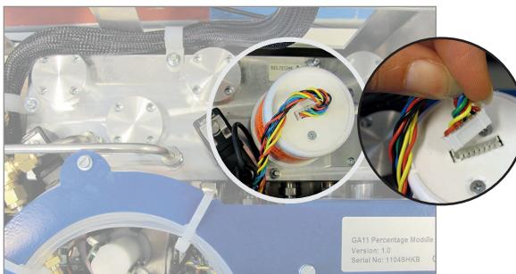
3. Screw out the sensor anticlockwise.
