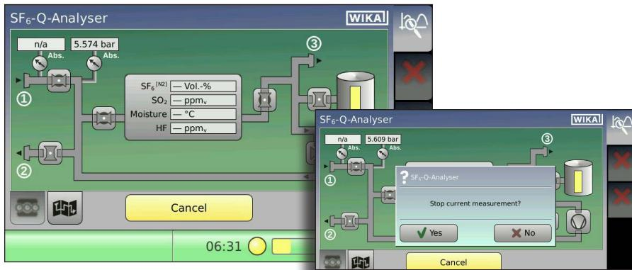
2. Select the gas compartment for pumping the measuring gas back (only available when the "pumping back" function is selected).
