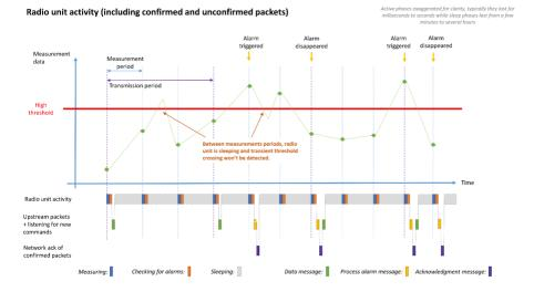
It shows that, in practice, a radio unit sleeps most of the time and wakes up only for short moments in order to assess the measured value, check if user-defined alarm conditions are matched or not, and periodically send and receive data from the LPWAN network.
