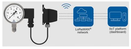
The protocol was designed to be compact in order to minimise the energy consumption (for longer battery life) and also use the shared radio spectrum more efficiently to enable more instruments to be connected to a given network.
