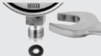
If the pressure instrument is positioned lower than the pressure test connection, the tailpipe has to be rinsed thoroughly prior to fitting the gauge to remove all foreign substances.
