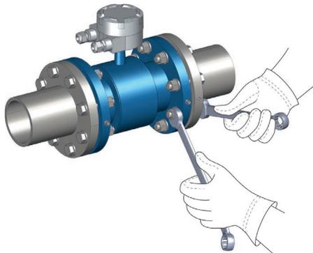
Fig. 33: Flange tightening
