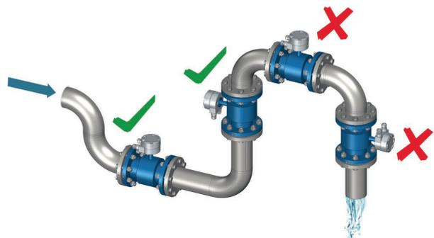
Fig. 24: Incorrect installation
