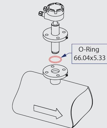
Insert the O-Ring gasket in the sensor stem.
