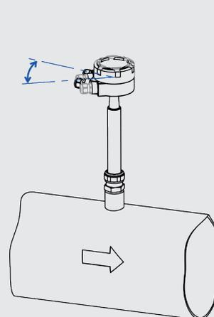
Adjust the alignment of the sensor in relation to the pipe (with an accuracy of  $\pm 2^\circ$ ) and the insertion depth.
