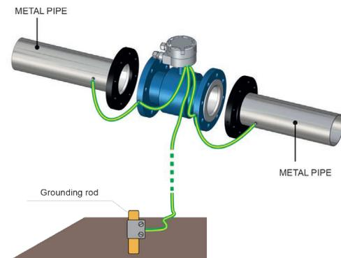
Fig. 47: Grounding of sensor on metal pipes
