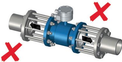
Fig. 26: Incorrect fixing
