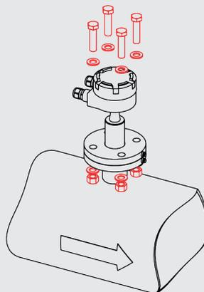
Insert the fixing bolts to secure the sensor flange to the flanged sleeve attached to the pipe.
