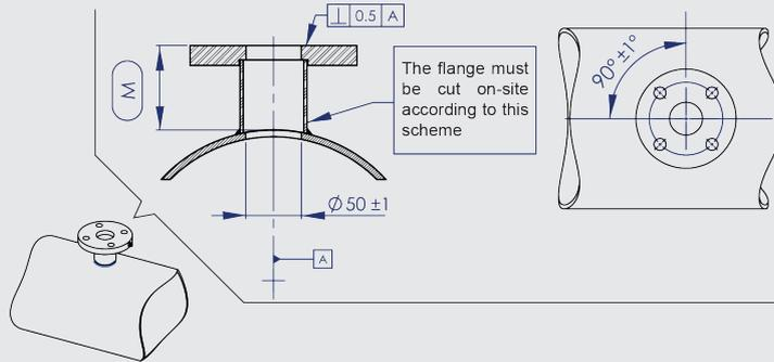
Prepare the flanged sleeve for assembly by cutting it to length **M** and weld it to the pipe, taking into consideration the following:
