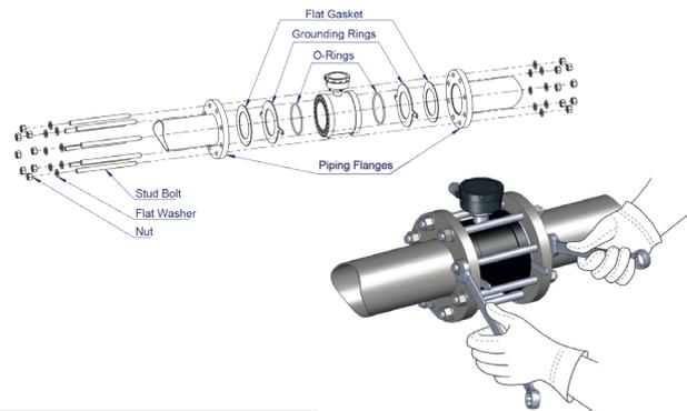
Fig. 34: Flange tightening
