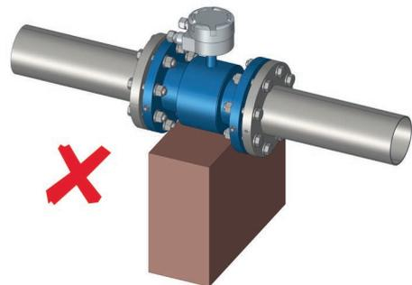
Fig. 31: Incorrect installation
