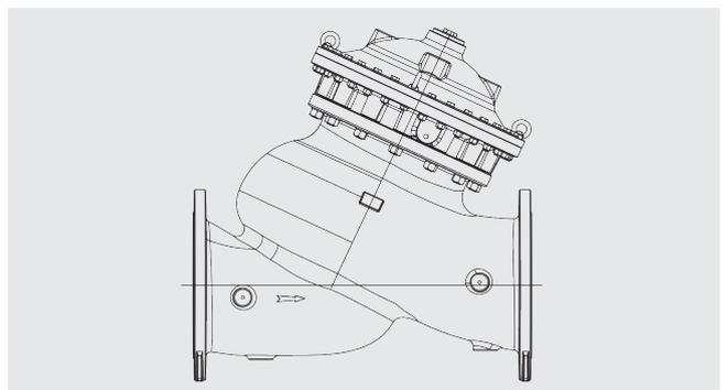
Fig. 38: Example of pressure control valves
