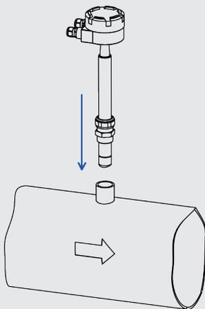
Insert the sensor into the threaded sleeve, taking care not to damage the measuring head.
