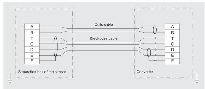
**Fig. 53: Standard double-shielded cables - C028**
