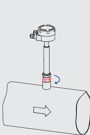
Tighten the nipple on the sleeve. Use the PTFE tape to ensure water tightness.
