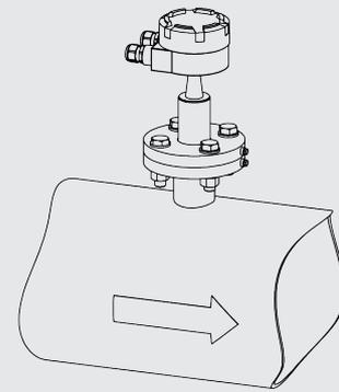
Tighten the bolts to block the position of the sensor.
