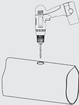
Drill in the installation position. The hole must have a minimum diameter of  $\varnothing 40$  mm in order not to interfere with the sensor head.
