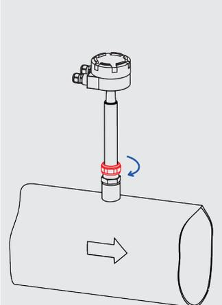
Tighten the upper ring nut of the nipple to lock the sensor in place.
