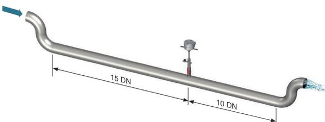
Fig. 14: Installation of Insertion Sensors on U-shaped tube
