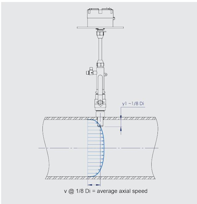
Fig. 57: Operating principle
