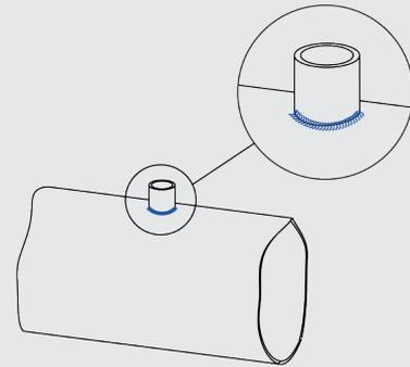
Weld a 1"1/4 GAS threaded sleeve to the pipe, centering it correctly on the hole.
