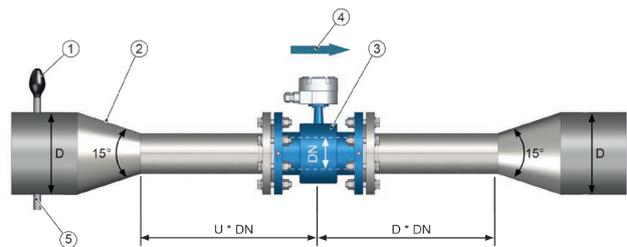
**Fig. 43: Installation on pipes with diameter reduction**
