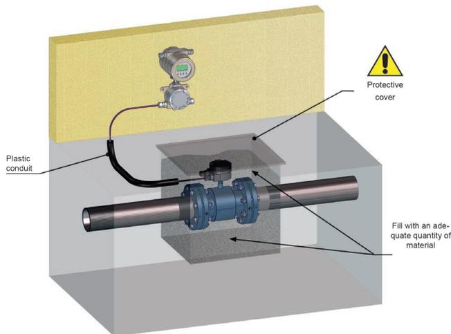
Fig. 35: Underground installation
