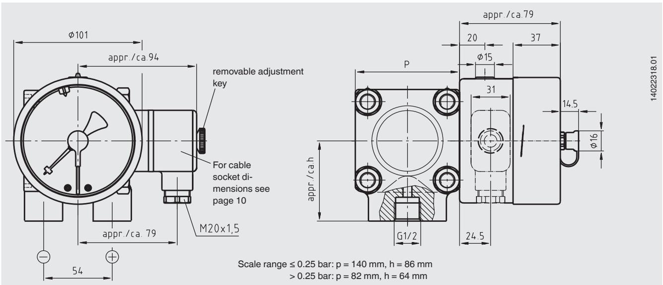
**switchGAUGE model DPGS43HP.160 with switch contact model 851.3**
