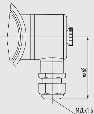
Only use cable with a diameter of 5 ... 10 mm
