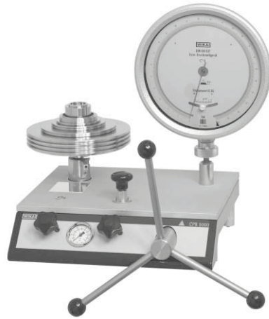
Pressure Balance CPB 5000 with device under test
