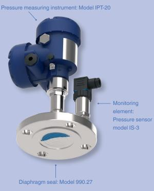
Pressure gauges, pressure sensors, pressure switches or process transmitters are suitable as measuring and/or monitoring elements.
