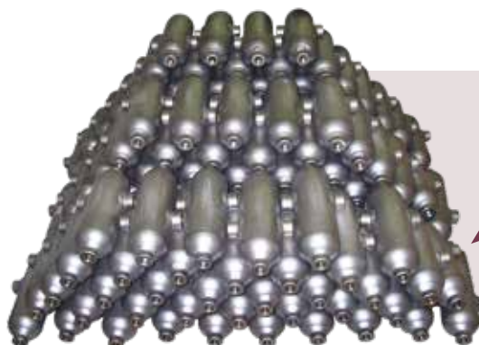
Condensate and seal pots are used as a barrier between the main line and the secondary instruments in the flow and pressure measurement of liquids, steam, or other vapours that can affect secondary instruments.
