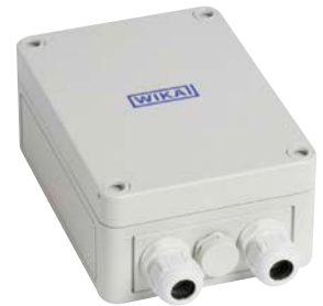
Many applications have a large distance between the measuring point and the read-out unit. A cable box outside the measuring point is an affordable way to bridge this distance. The box takes the high-quality connecting cable of the submersible pressure sensor and connects it to an inexpensive standard cable for onward signal transmission. | © WIKA
