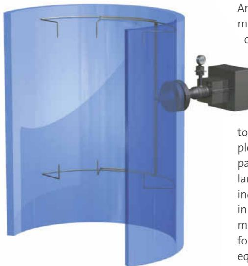
**Routing of the thermocouples within the reactor**
