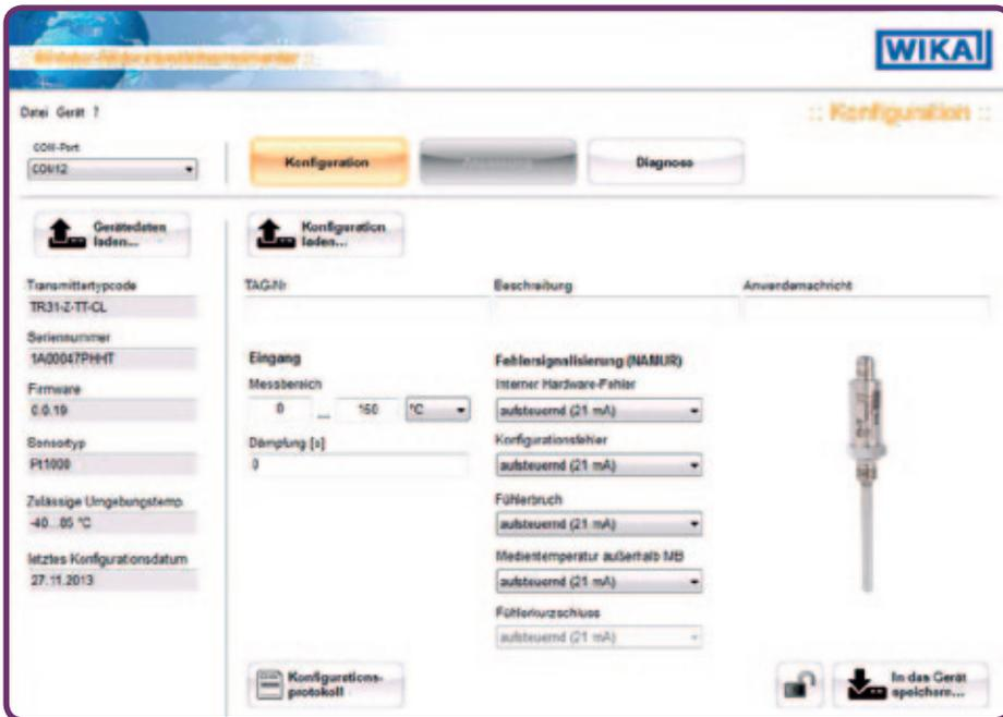
**02** Individually parameterisable for integrated transmitter with free PC configuration software WikaSoft-TT
