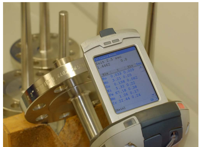
PMI test: X-ray fluorescence analysis of the thermowell stem
