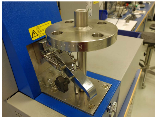
PMI test: Spectrographic analysis on a model TW10 flanged thermowell
