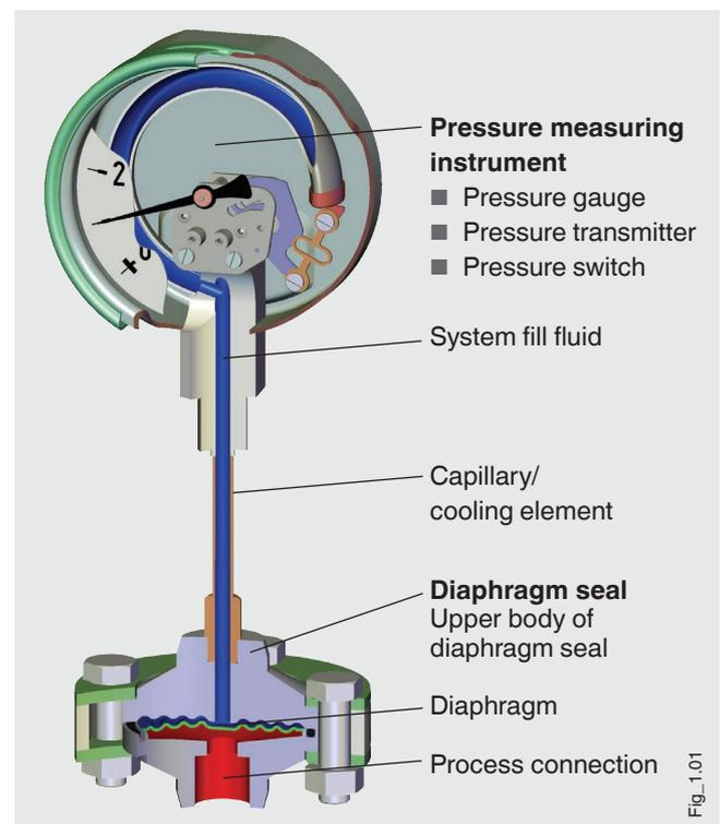
If the diaphragm is leaking, the system fill fluid can enter the medium. For food processing applications, it must be approved for contact with food. In selecting the fill fluid, the factors of compatibility, temperature and pressure conditions in the medium are of crucial importance. A variety of fluids are available which can cover the temperature range from -90 °C to +400 °C (see table "System fill fluids").
