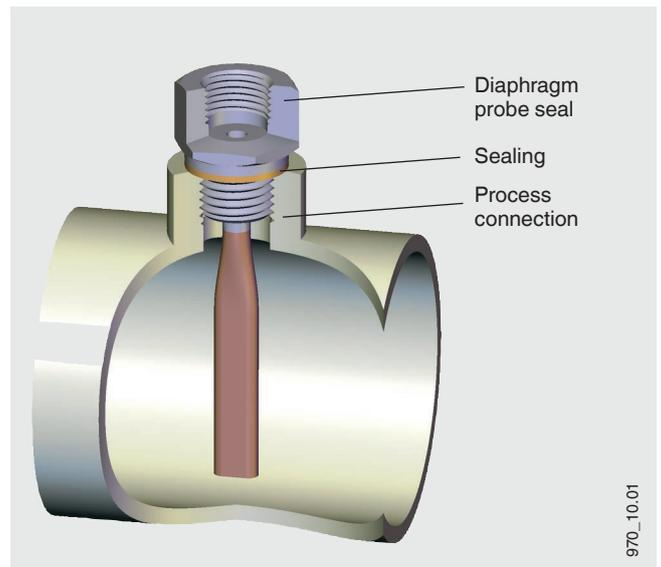
The standard material for diaphragm seals is stainless steel 316L. For the wetted parts, a wide range of special materials are available for almost all diaphragm seal designs.
