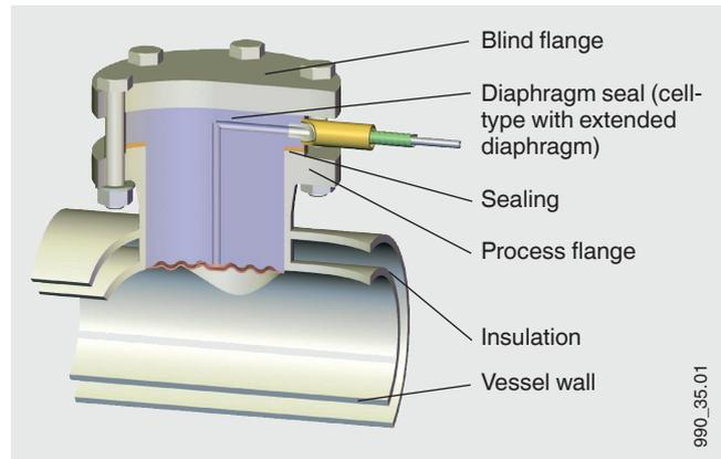
With diaphragm seals, pressures of up to 600 bar can be covered, with normal temperature limits at +400 °C.
