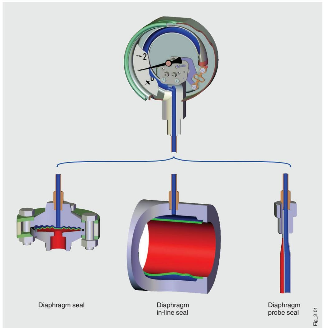
The decision for one diaphragm seal over another depends on both the specifications as well as the installation options and requirements of each specific measurement problem.
